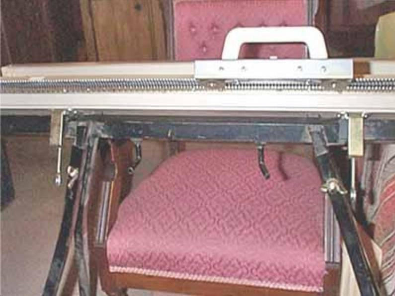
**Another view of the underside - everything clamped down. There is very little extra space on the tilted bars so be sure you get your machine clamps adjusted right to be equal on both sides of the bars that tilt.**
