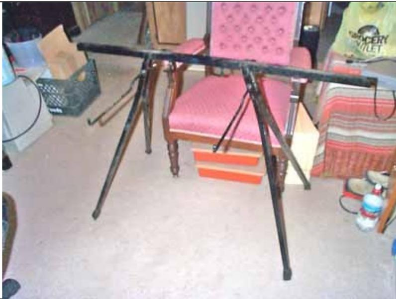
**Backside of stand - these two long bars sticking out are what holds the knitting machine's case lid so you can use it to hold yarns, tools or whatever.**
