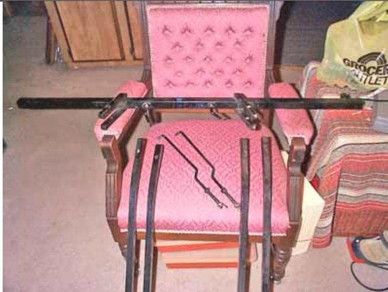
**Parts you should have - 4 legs, 1 center bar, 2 case lid bars. That's it! Very simplistic knitting machine stand to put up. It's rather portable too.**
