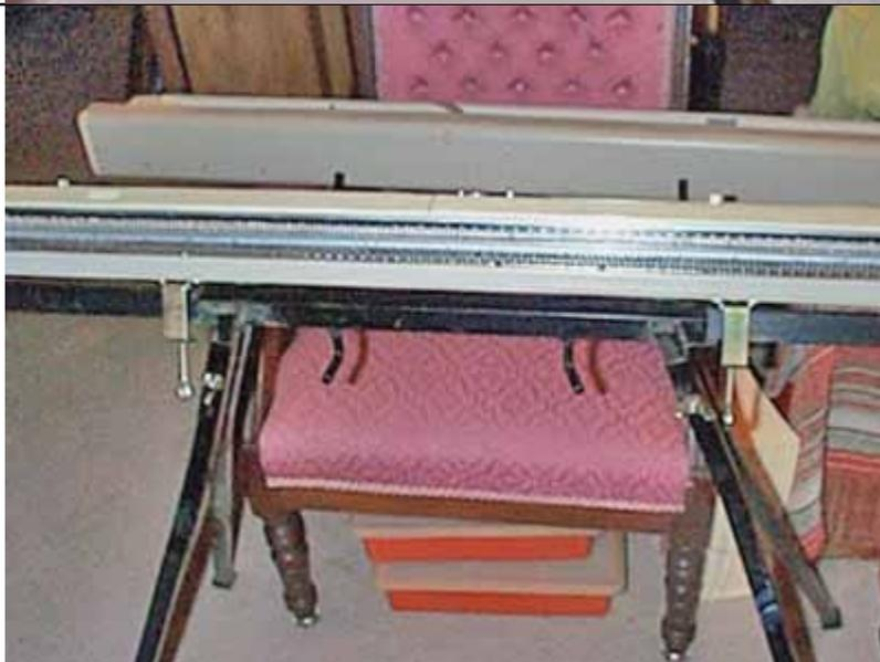
**Machine is now clamped onto the stand. The clamps are on the two OUTER bars of the stand. Now you need to adjust those two 'L-Shaped' levers to tilt the machine back. Depending on the weight of your machine, this may be a TWO PERSON JOB !!**
