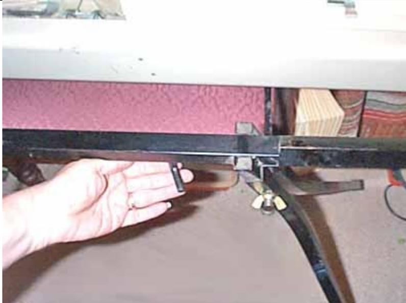
**These are the "L" shaped levers that screw in to tighten, out to loosen so the two sides will tilt back. The center portion of the stand remains untitled.**
