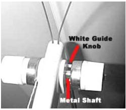
Pull the metal disk outward and you will see the metal shaft of the tension unit and you will also see a little white knob behind it. The yarn needs to go BETWEEN those two. It's very easy to slip it in there.
