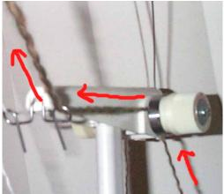
The arrows show the sequence of the thread up through the mast tension dial unit, out toward the front and through the little metal loop then it will go up to the loop at the end of the wire. See the next picture.
