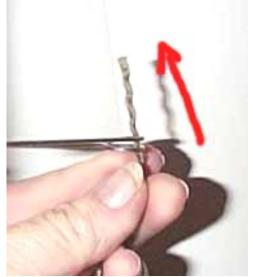
Place yarn on floor or on the table at the base of the mast. Put yarn end UP through eye of triangular guide.
