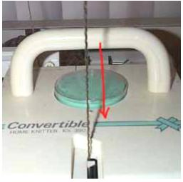
After the yarn is through the metal loop at the end of the wire, bring it down and thread through the machine.
